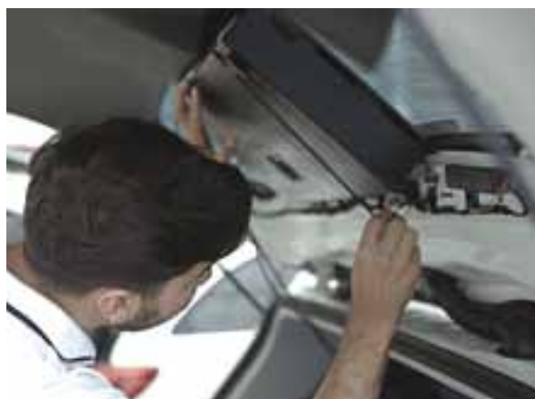
Three boxes were mounted into the back and into the side windows of each measurement car in order to support twelve smartphones per car.
